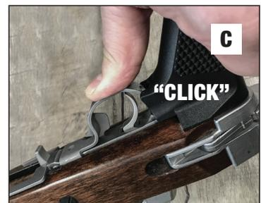
6. Cycle the slide handle and safety a few times to be certain the components are correctly assembled. Put the safety back "ON." Reinsert an empty magazine and fully withdraw slide. The bolt should lock open automatically.
