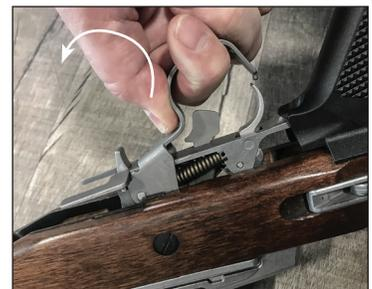
6. You can now remove the barrel/receiver assembly from the stock by lifting the rear of the assembly out of the stock and then pulling the stock rearward out of engagement with the gas block.
