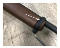
4. Position the safety so an equal amount of the button is exposed on each side. If the safety is not in the middle when the barrel-receiver assembly is inserted into the stock, the stock will be damaged.
