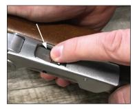
5. With your B-TM stock in the fully extended position, insert the barrel-receiver assembly downward into the stock. Be careful the two receiver cross pins and bolt stop pin do not fall out.
