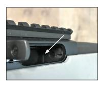
4. Position the safety so an equal amount of the button is exposed on each side. If the safety is not in the middle when the barrel-receiver assembly is lifted out of the stock, the stock will be damaged.
