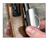
6. With the barrel-receiver assembly in place, insert the take-down screw you removed earlier to the underside of the B-TM wooden stock and tighten using the appropriate size Allen wrench.
