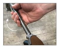
7. Slide the barrel band over the barrel and onto the B-TM stock and tighten the screw.
