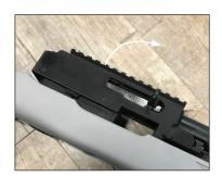
3. Use an appropriate size Allen wrench to loosen and remove the take-down screw on the underside of the wooden stock. Set the take-down screw aside for use when installing the barrel/receiver assembly into your B-TM Folding Stock. (Step 6 on back)
