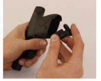
**Step 2**Insert the locating pin at the front of the Compact Magwell into the magazine release sping notch in the pistol frame. Do not adjust the depth of the locating pin.
