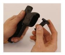
**Step 1**Orient the Compact Magwell with the finger groove toward the muzzle so that the clamp mechanism aligns with the pocket in the backstrap.
