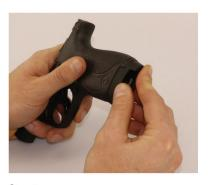
**Step 3**With the locating pin fully engaged push the clamp mechanism into the backstrap pocket with enough force to close the gap between the frame and the Compact Magwell.
