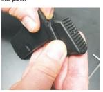
**Step 5** Hold the retaining plate inside the magazine tube while sliding the +2+ Magazine Extension from the front to the rear.
