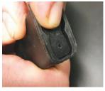
**Step 4** Press the replacement retaining plate into the magazine tube.
