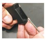
**Step 2** Slide the factory base plate forward and off of the magazine body, then remove the existing retaining plate.
