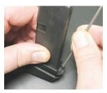
**Step 7** Once the +2+ Magazine Extension is move fully forward, use the 7/64 hex wrench to install the cap head screw. You might want to use a drop of blue thread locker here.
